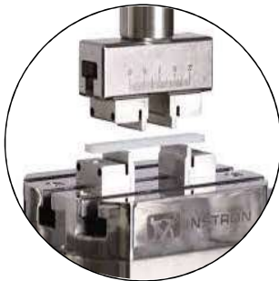
Bending Load Testing facility – 5 Tons
